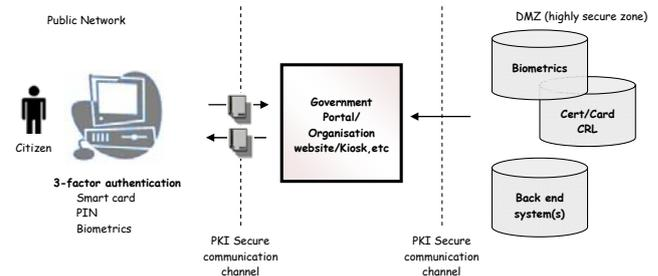
Fig. 8 conceptual model for electronic authentication
